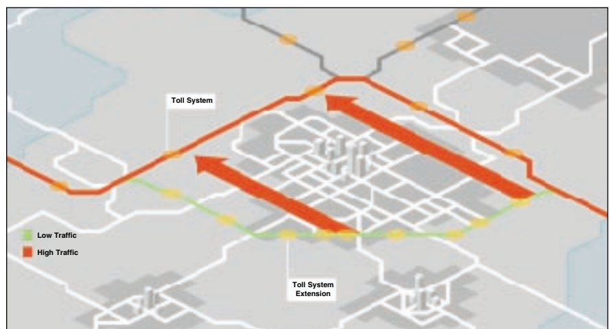
Solution of traffic diversion by extension of GNSS toll system
